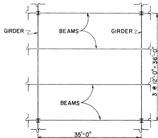
Fig. 1. Plan view of floor system
