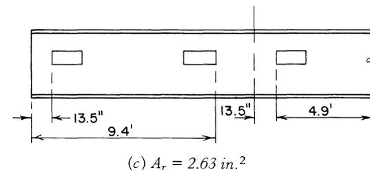
Fig. 8. Permissible opening locations for girders
