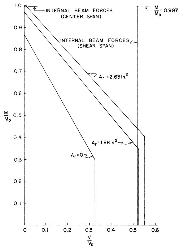
Fig. 7. Girder interaction diagrams
