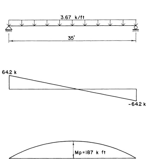
Fig. 3. Floor beam loading, shear, and moment diagrams
