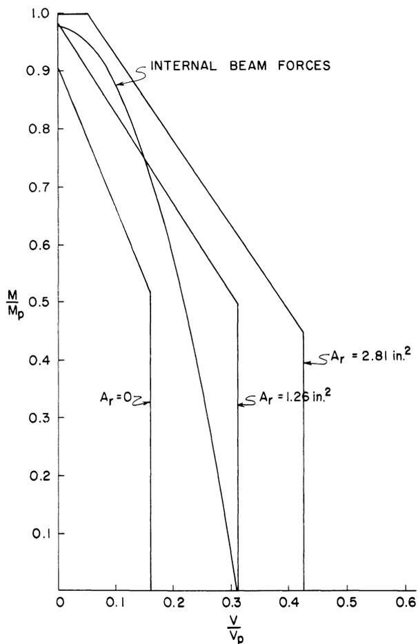
Fig. 4. Floor beam interaction diagrams
