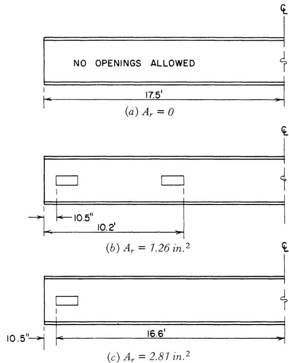
Fig. 5. Permissible opening locations for floor beams
