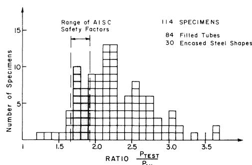
Fig. 1. Axially loaded composite columns
