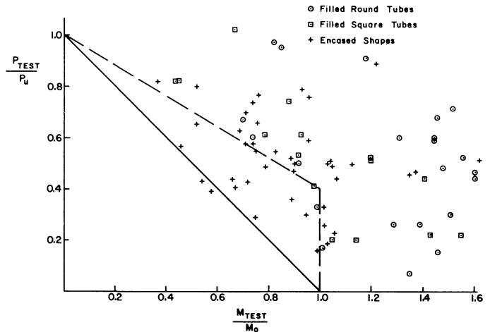
Fig. 2. Eccentrically loaded composite columns
