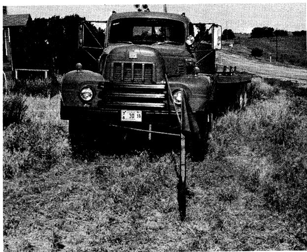
Fig. 8. Test truck, showing tell tale guide for driver
