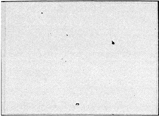
Fig. 9. Unetched photomicrograph of microscopic inclusions as cast in steel ingot (magnification 100X)
