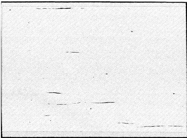
Fig. 10. Unetched photomicrograph of microscopic inclusions elongated during rolling (magnification 100X)
