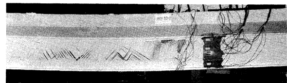
Fig. 8. View of Beam 32 at the end of the test. The separation at the right end and the absence of concrete crushing at midspan can be noted. This is a typical view of specimens with shear failure. The A514 portion of the web shows no yield lines. Web buckled after the maximum load was reached. Yielding due to buckling can also be seen.
