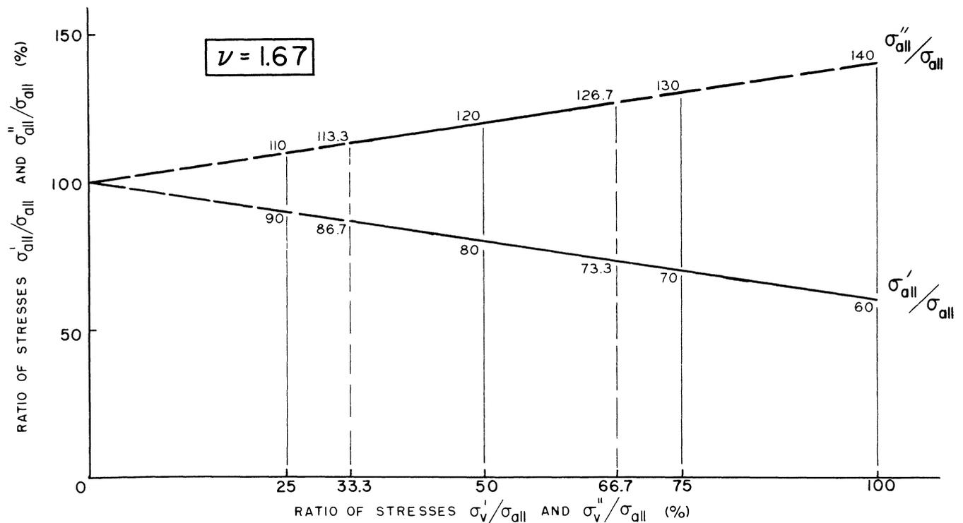
Fig. 3. Variations of allowable stress  $\sigma''_{all}$ ,  $\sigma'_{all}$  in prestressed structures designed according to modified allowable stresses.
