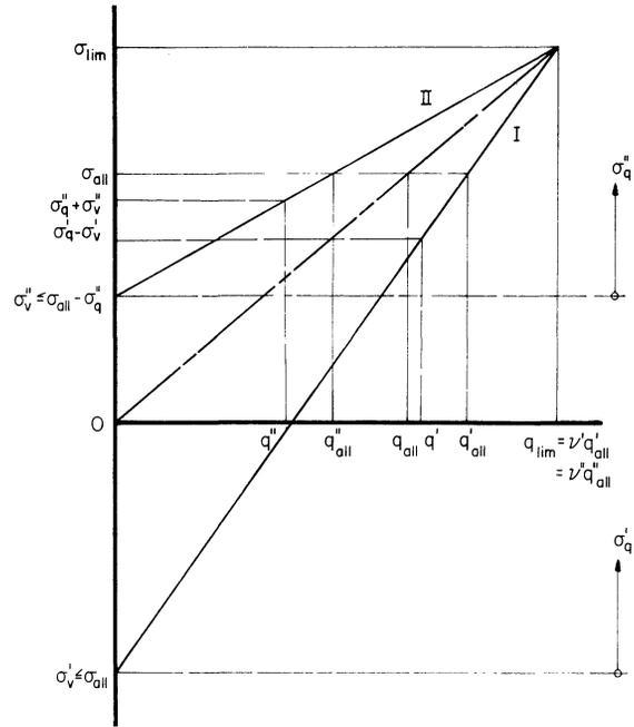
(b) ANALYSIS OF PRESTRESSED STRUCTURES ACCORDING TO ALLOWABLE STRESSES.
