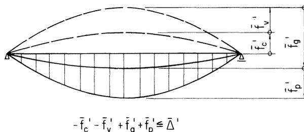
(b) TOTAL CAMBER LESS THAN DEAD LOAD DEFORMATIONS
