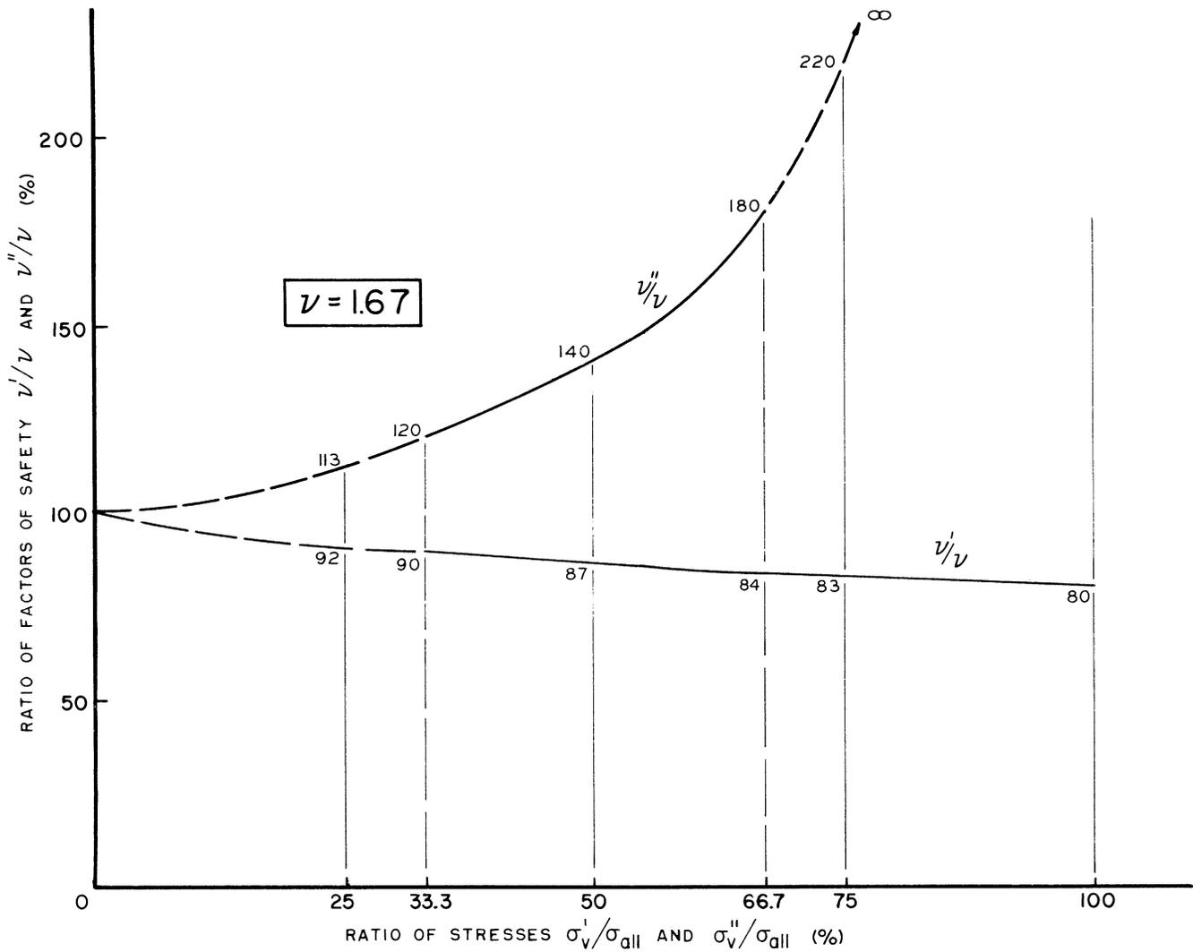
Fig. 2. Variation of safety factors  $\nu'$ ,  $\nu''$  in prestressed structures designed according to allowable stresses.
