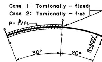
Fig. 9. Two-span continuous curved girders
