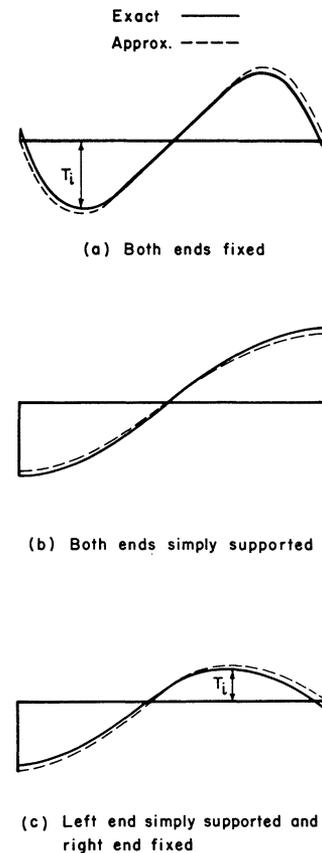
Fig. 7. Torsional moment diagrams showing effect of various end restraints in bending
