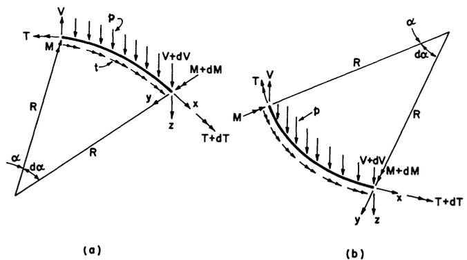
Fig. 1. Sign convention for external and internal forces
