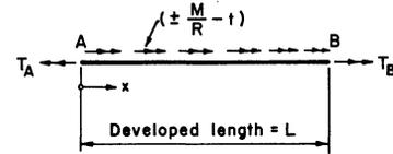
Fig. 2. Torsional loading on developed girder
