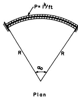
Fig. 5. Circular girder with fixed-ends
