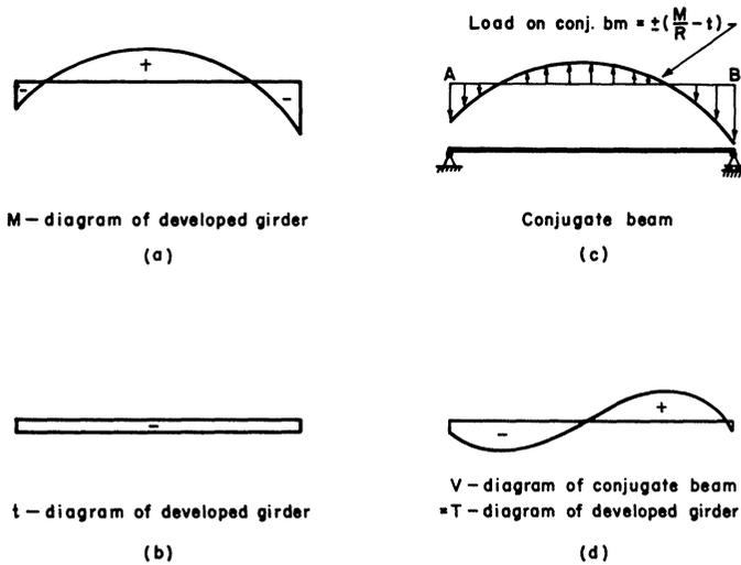
Fig. 3. Conjugate beam  $M/R$ -method
