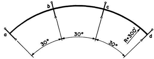
Fig. 8. Three-span continuous curved girder
