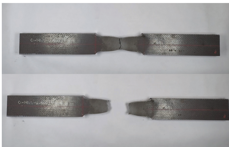
Fig. 3. Result of full-thickness tensile coupon testing.
