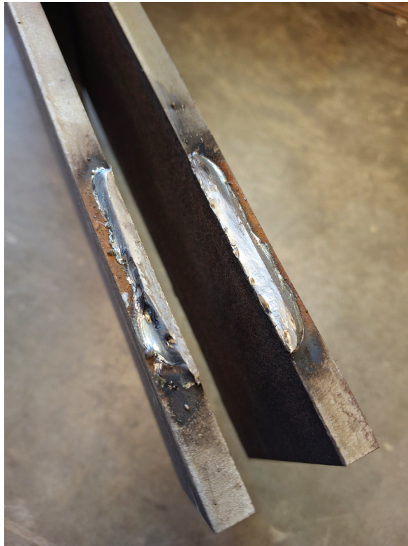
Fig. 14. Photograph of weld failure for specimen S42.
