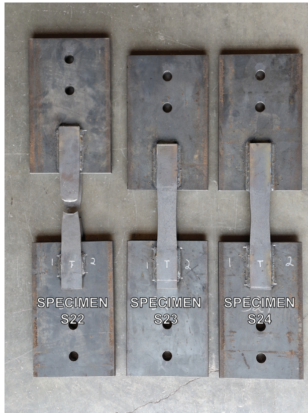
Fig. 12. Photograph of specimens that failed in the plate.
