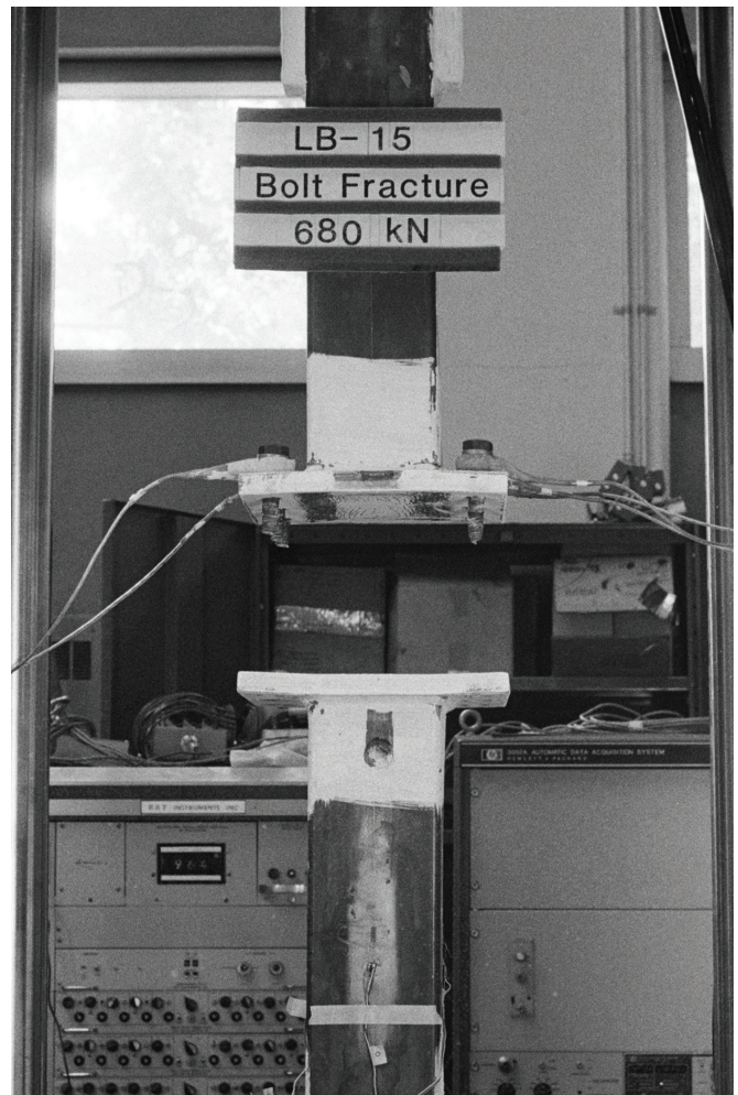
(b) Ultimate failure
