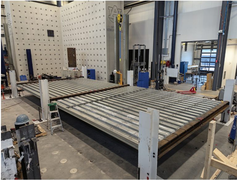
(a) AIBs supporting deep decking
