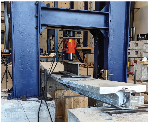
Fig. 11. Example composite beam test under loading and load time-history plot.
