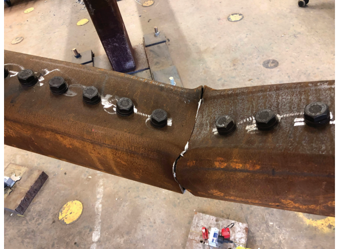
(b) Specimen 2 (flange yielding in compression)
