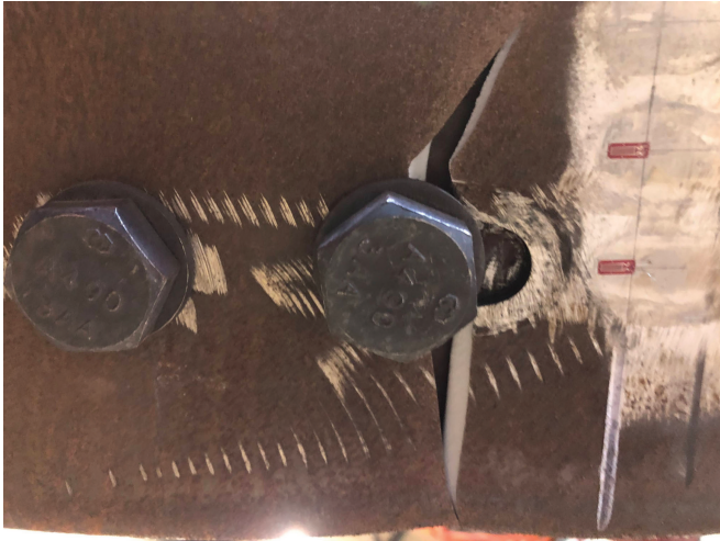
(a) Specimen 3 (HSS 7x7x \frac{1}{4} )
