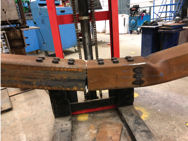
(a) Specimen 1 (compression flange buckling)
