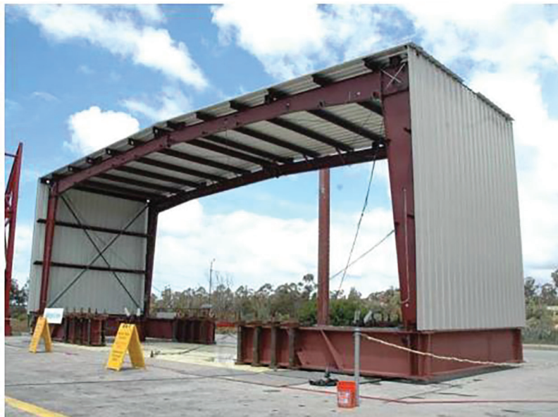
Fig. 1. Assembled specimen on shaking table (Smith et al., 2013).
