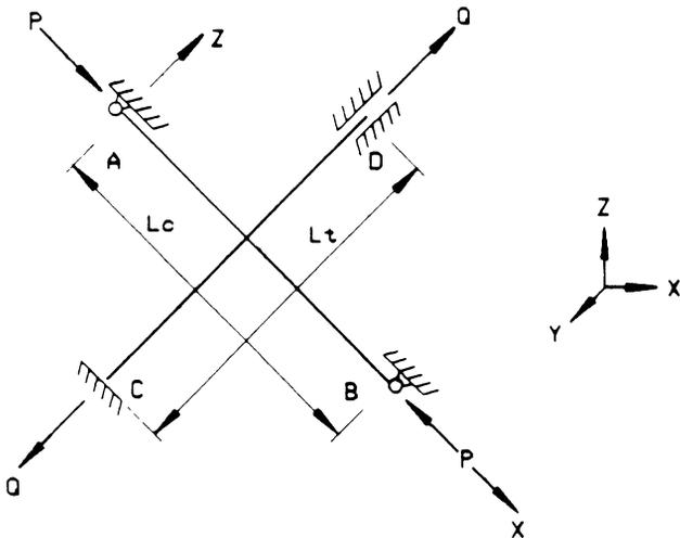
Fig. 3. Cross bracing with tensile brace built-in
