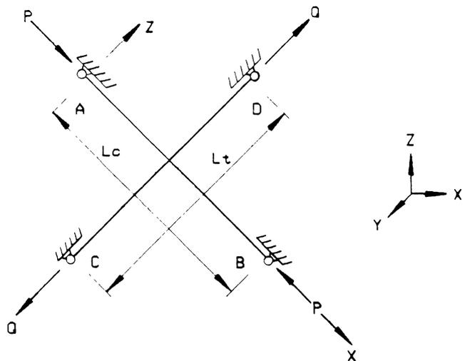
Fig. 2. Simply supported cross bracing
