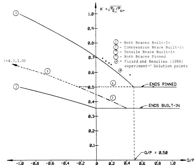
Fig. 7. Effective length factor for identical cross bracing of various boundary conditions
