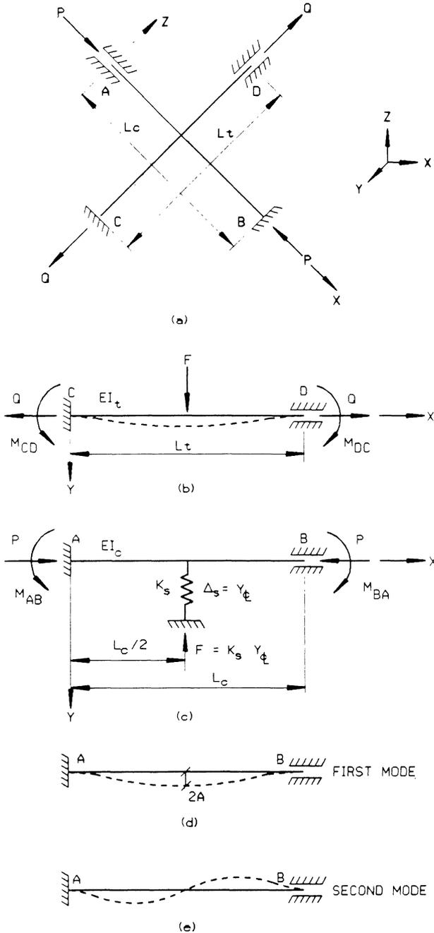
Fig. 1. Built-in cross bracing system
