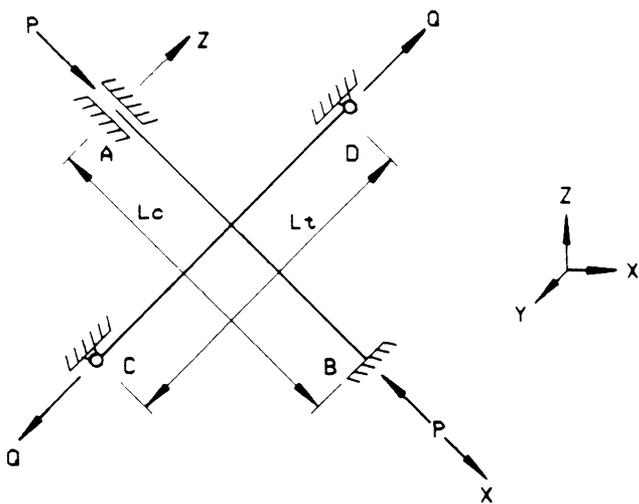
Fig. 4. Cross bracing with compressive brace built in
