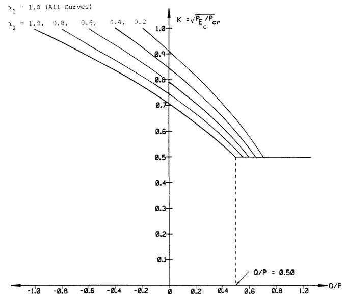
Fig. 6. Effective length factor spectra for simply supported cross bracing
