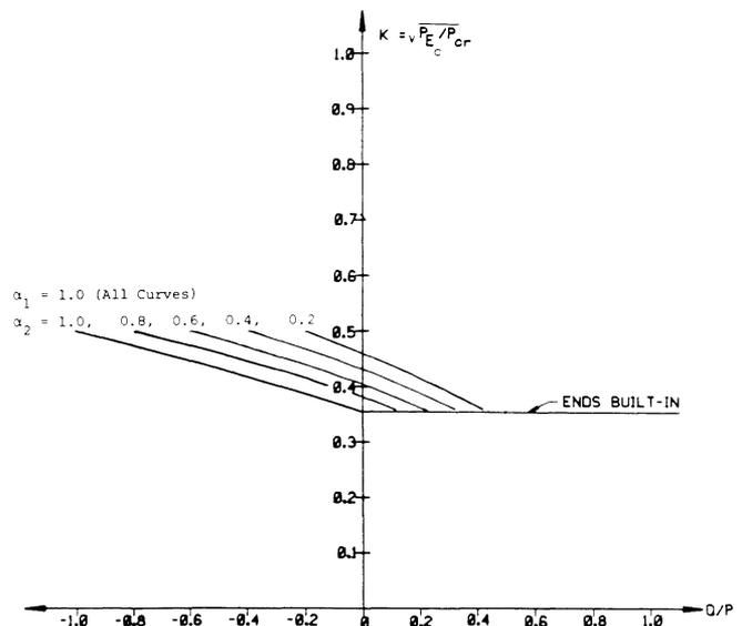
Fig. 5. Effective length factor spectra for built-in cross bracing
