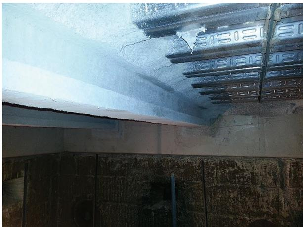
(a) Typical SFRM-protected beam (showing the longitudinal seam between slabs of adjacent specimens)
