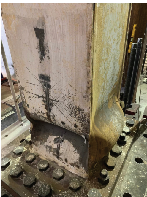
(a) Local buckling in the experiment
