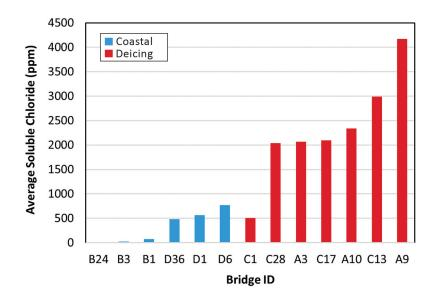
Fig. 6. Average soluble chloride concentrations for representative coastal bridges and highway overpasses in environments where deicing agents are used.
