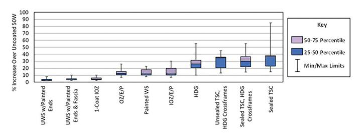
Fig. 3. Box and whisker plot of relative first costs of common corrosion protection systems (AISC, 2022).
