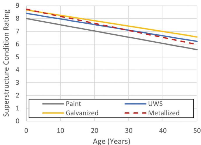
Fig. 2. Linear regression lines of condition versus age for various corrosion protection systems (not for extrapolation).
