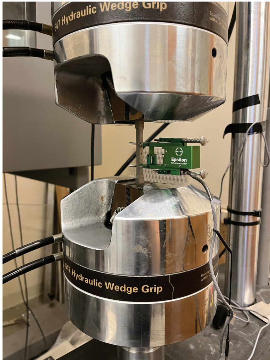
Fig. 2. Tensile coupon test setup.
