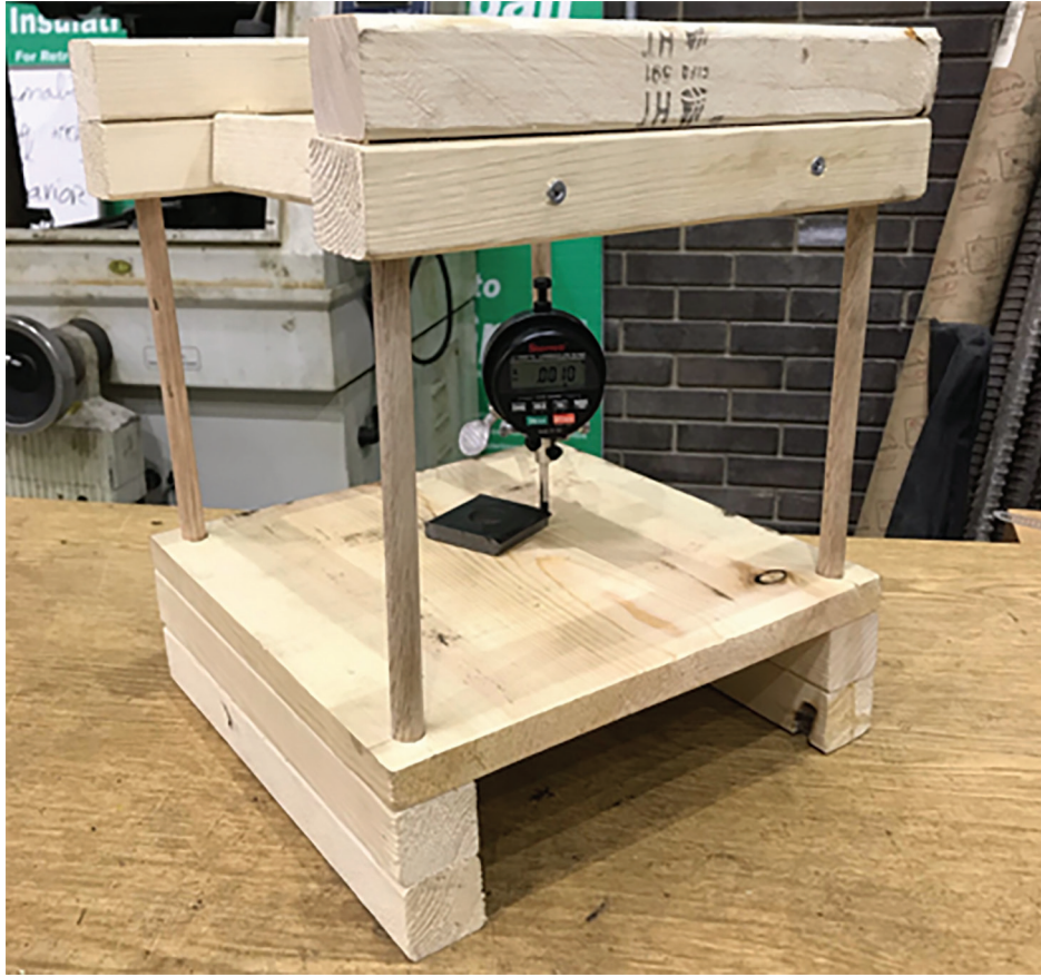
Fig. 5. Assembly of stage and affixed dial gauge.
