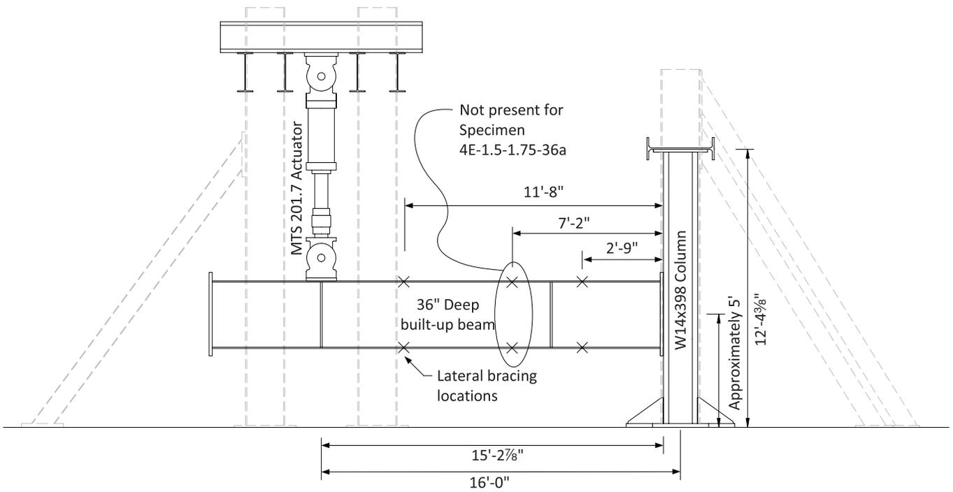
Fig. 2. Schematic of test setup.
