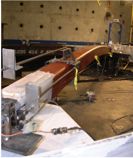
(a) Initial brace buckling
