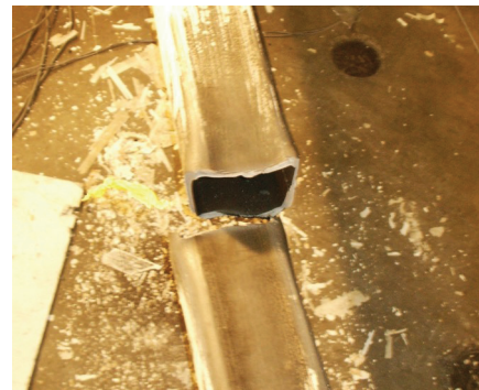
(f) Fracture after ductile tearing of most of cross section
