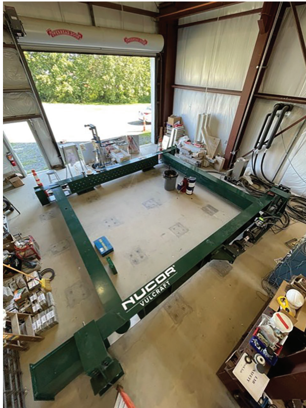
Fig. 5. Cantilever diaphragm testing rig at UMass Amherst.
