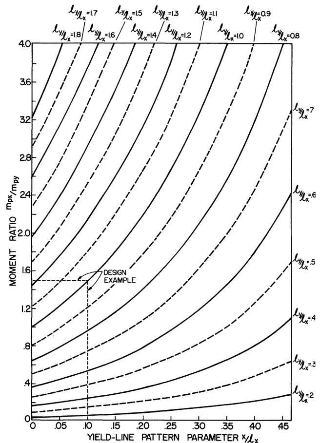
Fig. 4. Analysis and design curves for general rectangular grid
