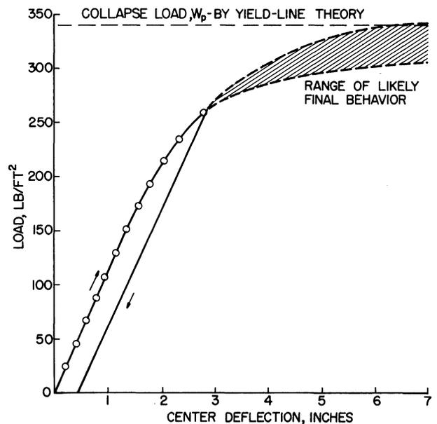
Fig. 7. Load-deflection curve for thread-through bar joist grid
