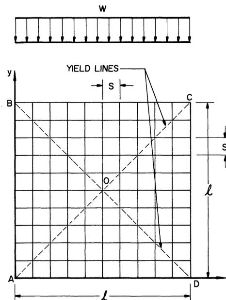
Fig. 1. Square grid and yield-line pattern for edge supports and uniform load
