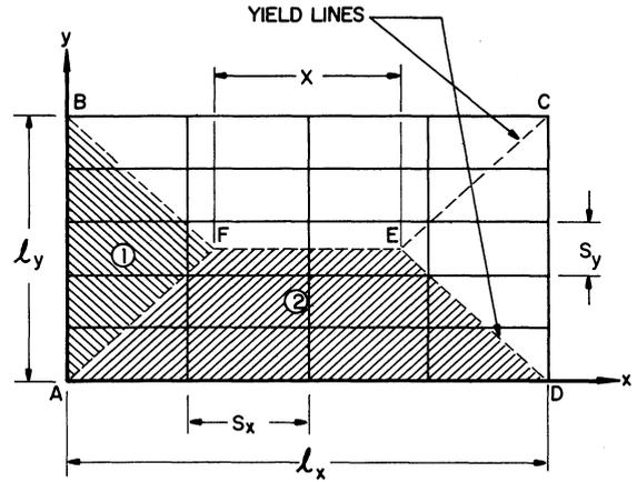
Fig. 3. General rectangular grid showing yield-line pattern
