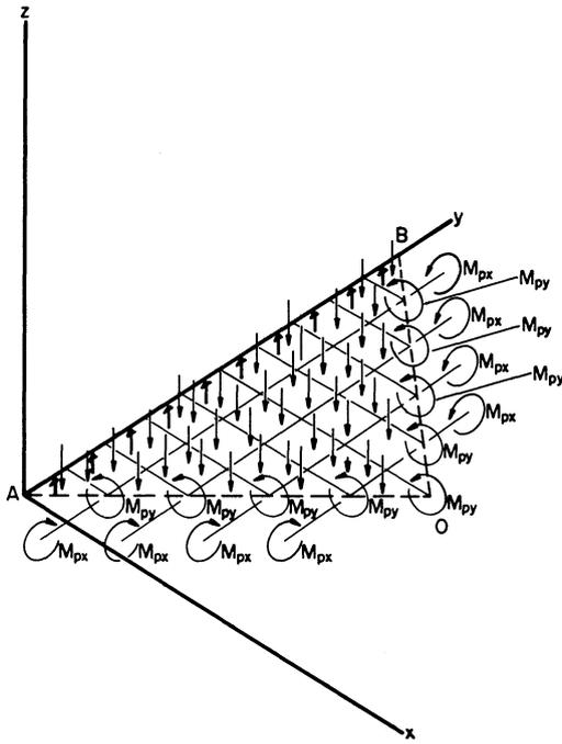
Fig. 2. Free-body diagram of segment ABOA of square grid
