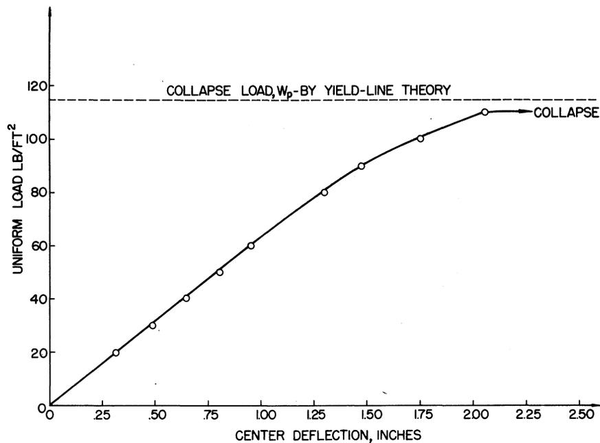
Fig. 6. Load-deflection curve for thread-through model grid
