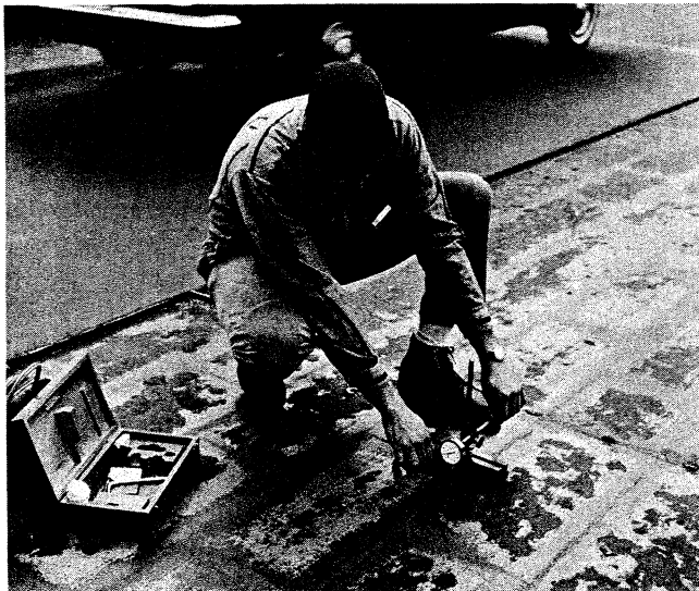
Fig. 4. Dial indicator measurements of typical deck surface condition. Corresponding profile is shown in Fig. 7a
