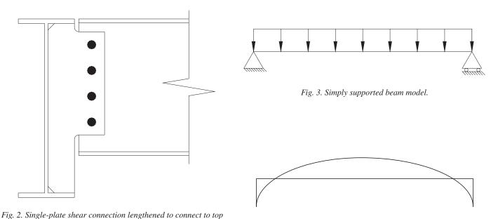
and bottom flanges of support. Fig. 4. Moments on a fixed-end beam.
