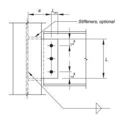
Fig. 9. General extended single-plate connection configuration.
