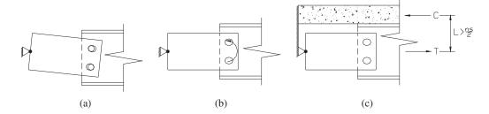
*Fig.* 7. Support rotation at short slotted holes. (a) Support restrained by bolts slipping into bearing. (b) Support restrained by slip resistance to moment. (c) Support restrained by slip resistance to tension and compression in slab.
