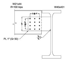
Fig. 1. Extended single-plate shear connection.
