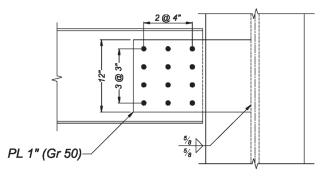
Consider a  $W16\times 26$  with a 100 kip (LRFD) end reaction (see figure). Find an extended single-plate shear connection to support the end reaction.
