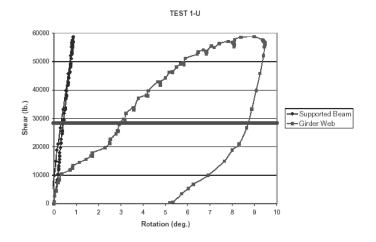
Fig. 8. Plot of shear versus rotation for the Sherman and Ghorbanpoor test 1-U.
