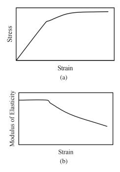
Fig. 5. (a) Stress-strain and (b) modulus of elasticity-strain curves for steel (based on tangent modulus).
