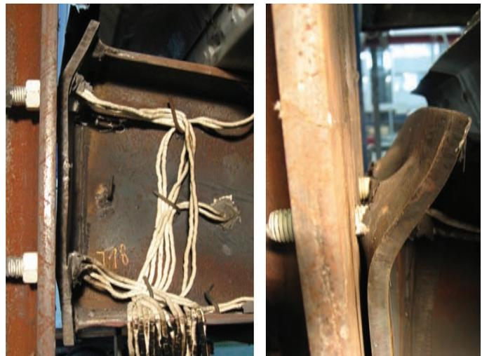
Fig. 16. Joint deformation at test FJ01.
