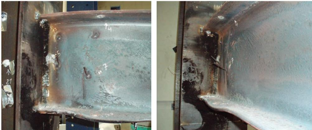
Fig. 21. Local buckling on the beam bottom flange and shear buckling of the beam web (joint Z2).
