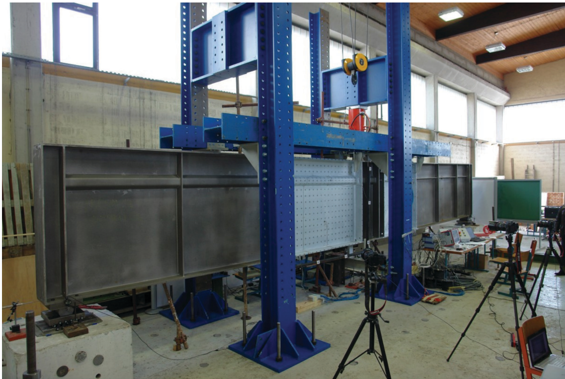
Fig. 6. Test setup for a large-scale plate girder. (Photograph courtesy of Professor Darko Beg)
