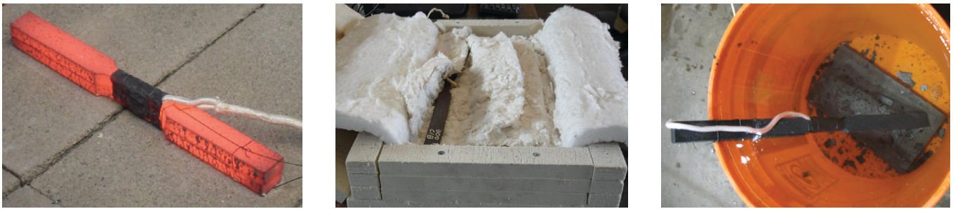
Fig. 3. Cooled-in-air (CIA), cooled-in-blanket (CIB) and cooled-in-water (CIW).
