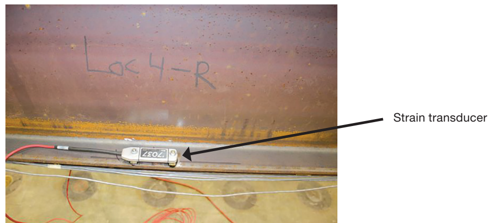
Fig. 12. Strain gage, Location 4.
