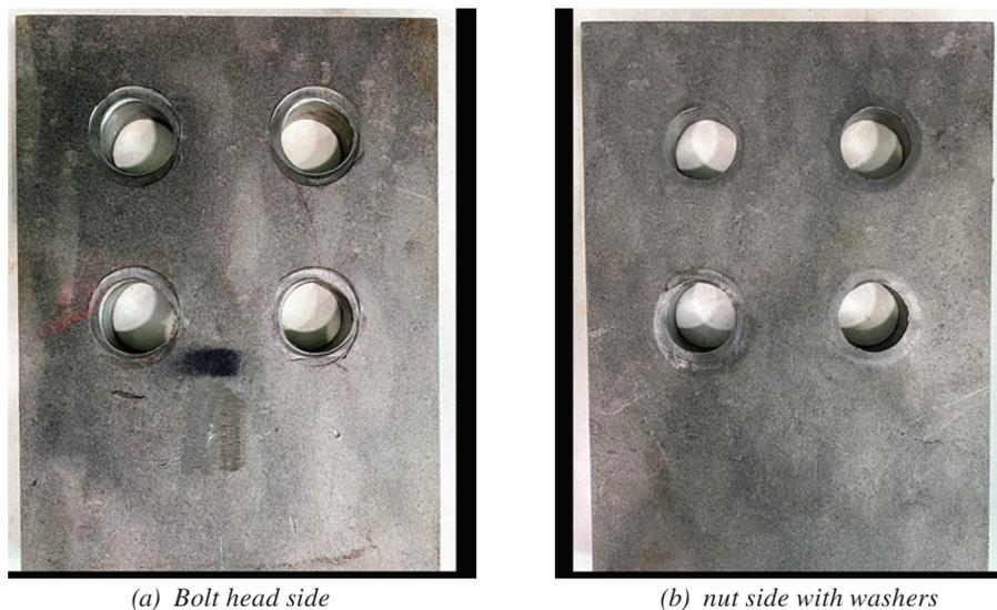
Fig. 12. Plate dents from 1 in. bolt specimens.
