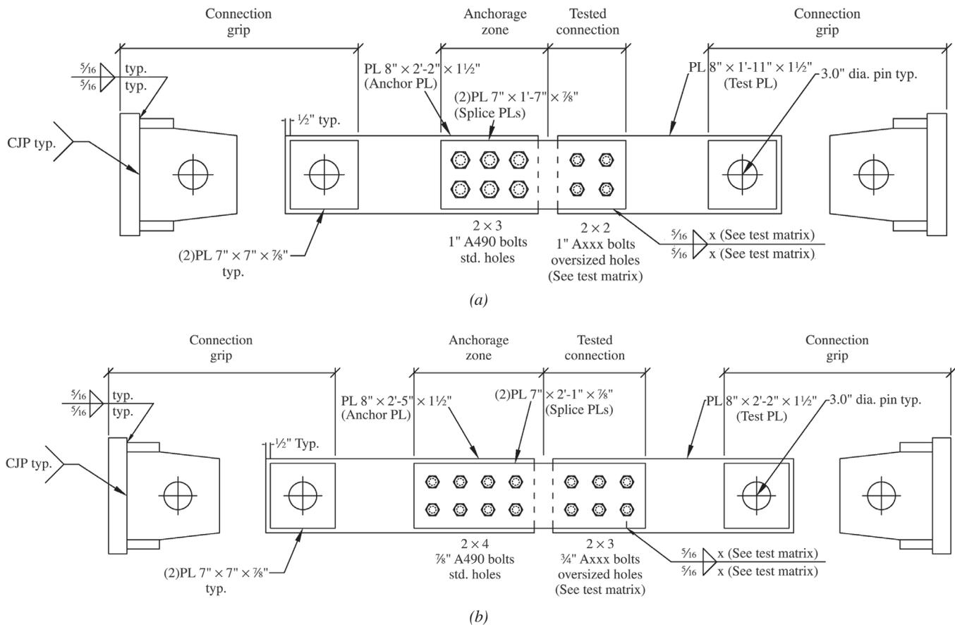
Fig. 1. Details of test specimens.
