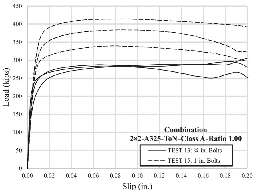
Fig. 11. Bolt size load-slip curve comparison:  $\frac{3}{4}$  in. diameter vs. 1 in. diameter.
