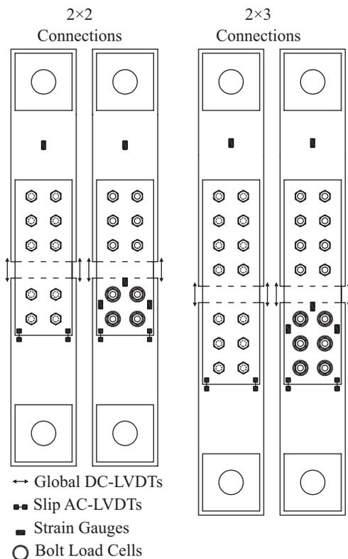
Fig. 4. Specimen instrumentation layout.
