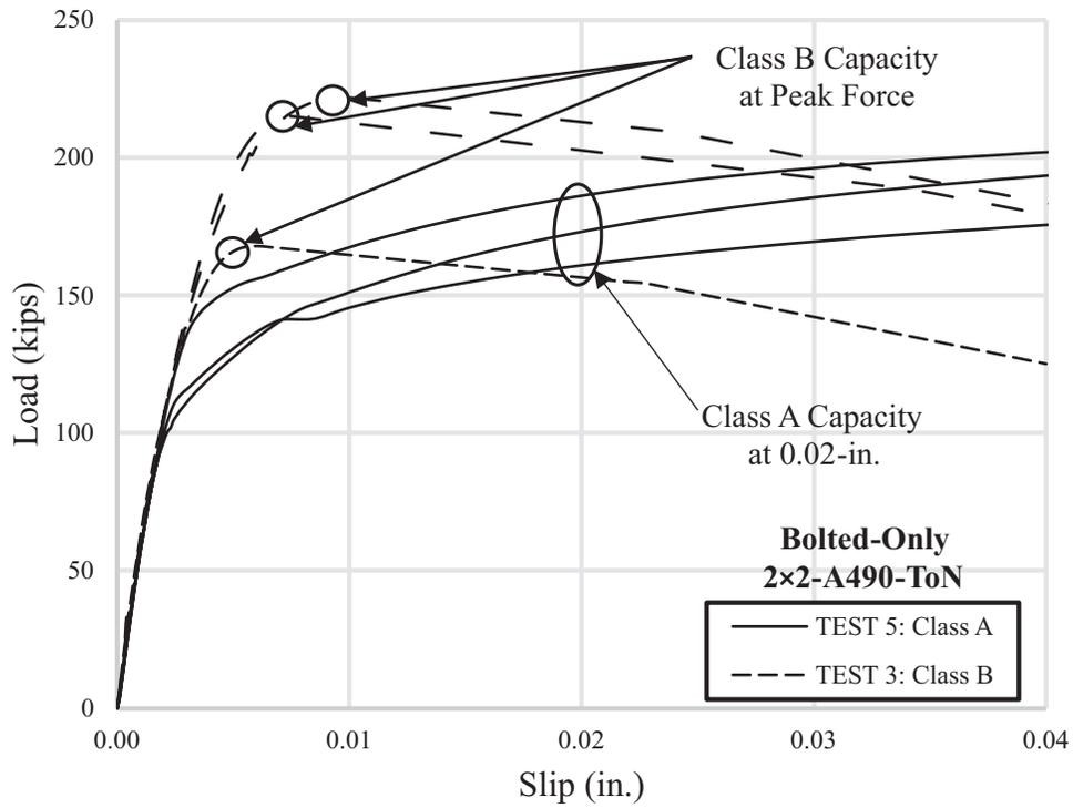
Fig. 6. Bolted-only experimental load-slip curves.
