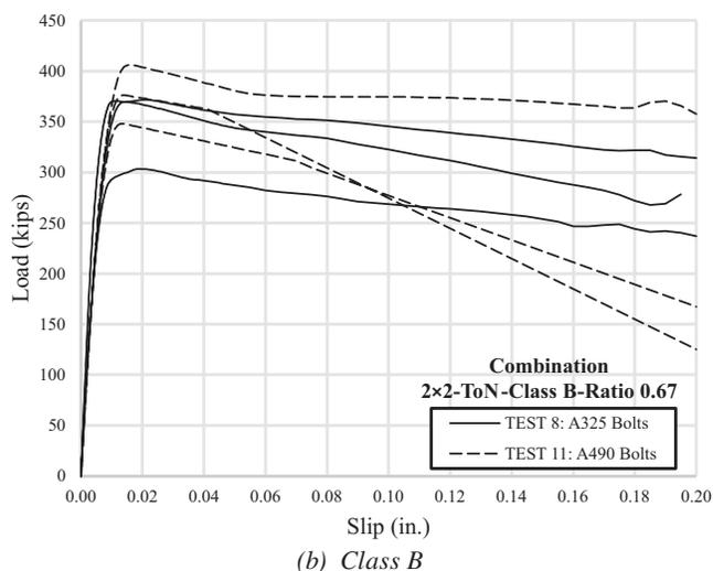
Fig. 13. Bolt grade load-slip curve comparison: A325 vs. A490.
