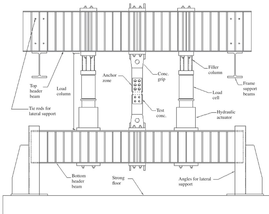
Fig. 3. Experimental test frame details.
