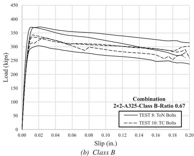
Fig. 14. Bolt tensioning method load-slip curve comparison: ToN vs. TC.
