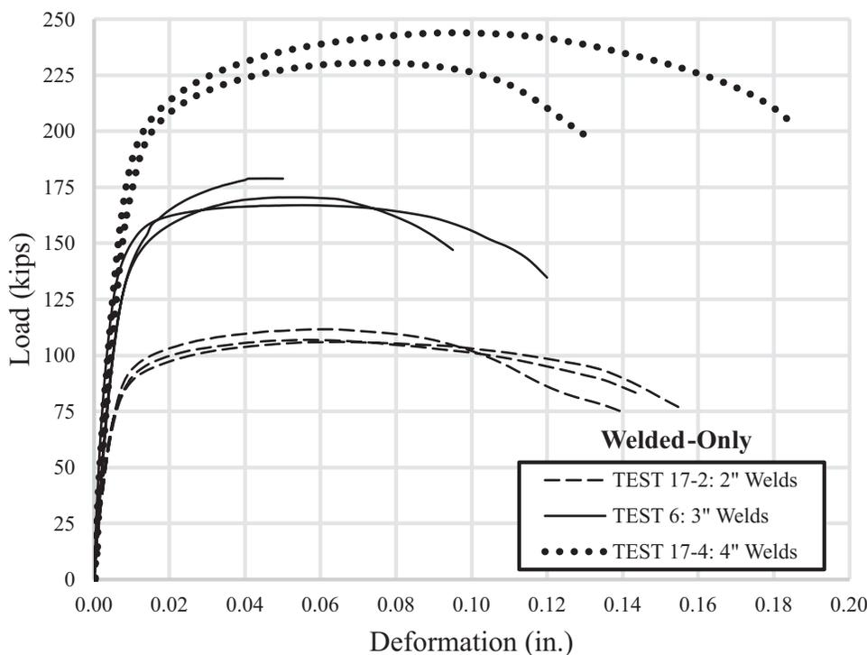
Fig. 7. Welded-only experimental load-deformation curves.
