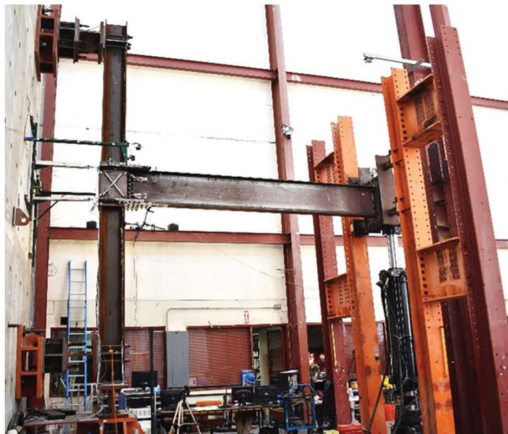
(b) Installed specimen (G1.1) and out-of-plane restraint at actuator
