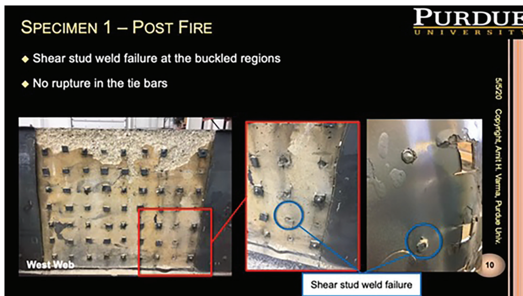
Fig. 5. Screenshot of video presentation on SpeedCore fire resistance experiments (Varma, 2021).
