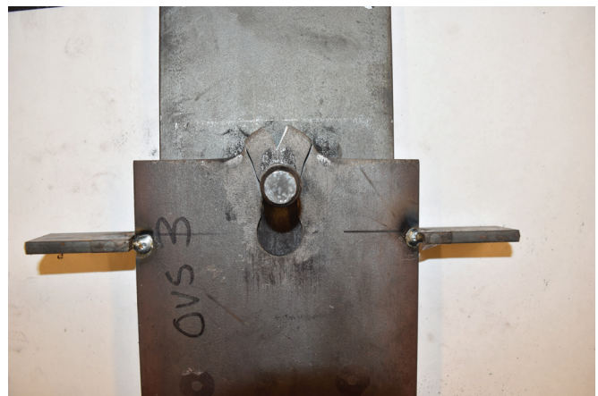
(b) Specimen OVS3 after testing
