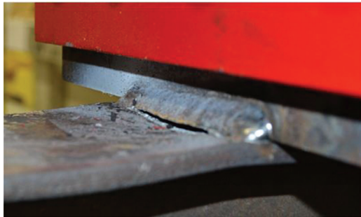
Fig. 16. Weld fracture of W16×31 ST-E6 after testing (side 1).
