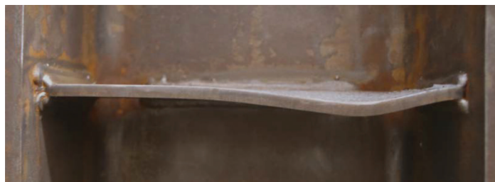
(c) Continuity plate buckling in experiment
