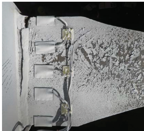
(b) Fracture in top flange CJP groove weld during test
