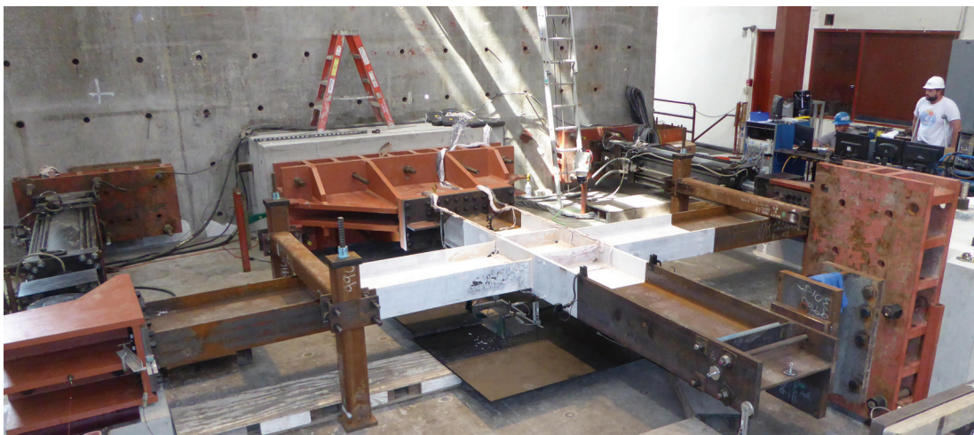
Fig. 2. Interior moment connection test setup.
