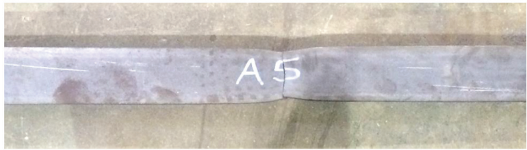
Fig. 9. Typical gross section fracture.
