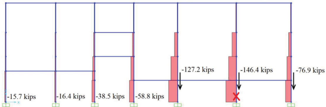
Fig. 12. Calculated axial load distribution for model B (with composite beams and no ribbed slabs) before the test column removal (under red cross).
