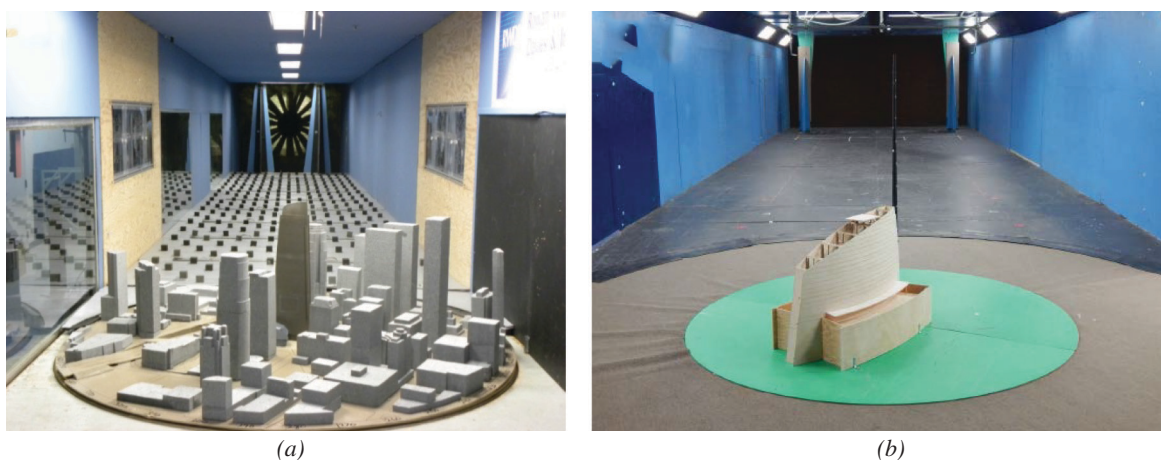
Fig. 3. Wind tunnel model of (a) tower and (b) spire.
