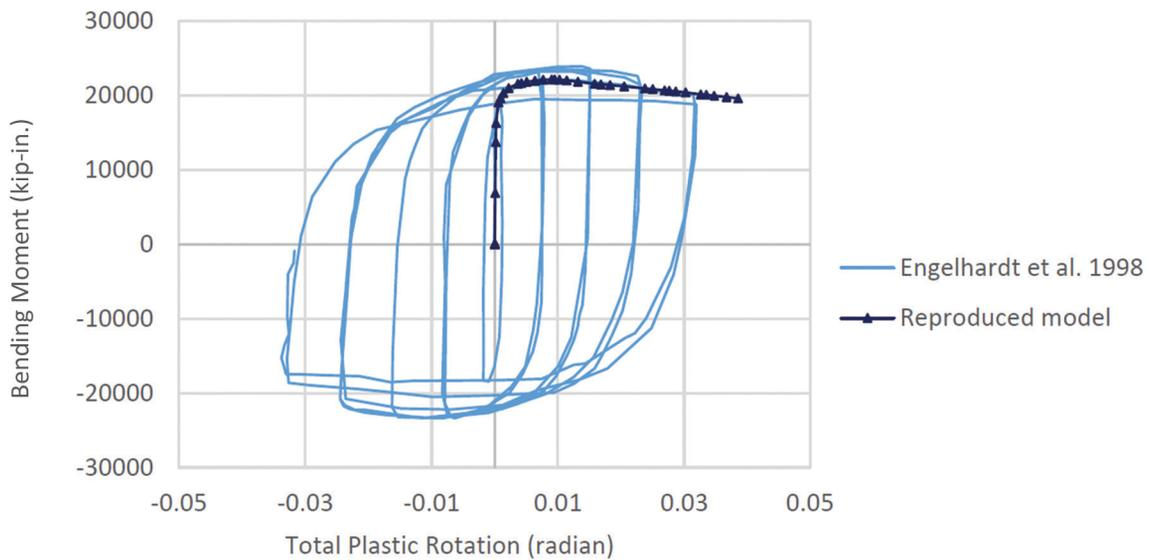
Fig. 1. Bending moment vs. total plastic rotation comparison.
