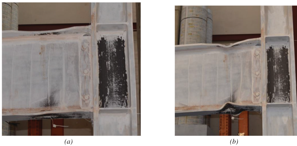
Fig. 8. Global view of specimen C2: (a) at 0.04-rad drift (second cycle); (b) at 0.07-rad drift (first cycle).
