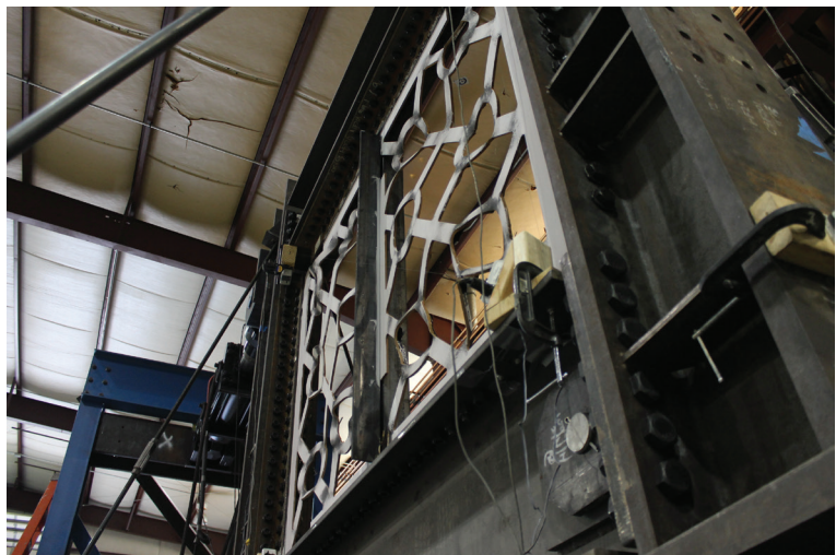
Fig. 8. Global shear buckling in fifth-story RS-SPSW specimen.
