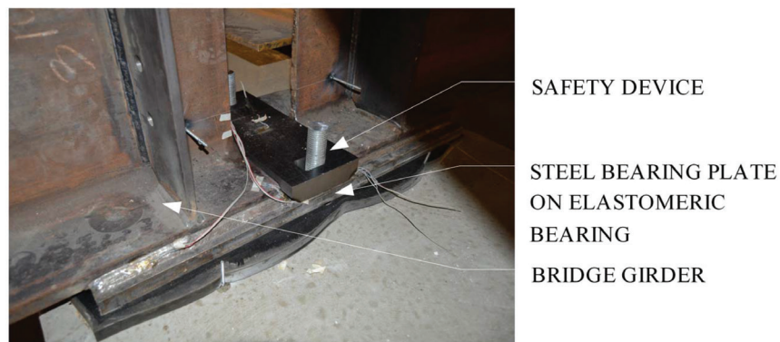
Fig. 12. Safety device at end of physical test.
