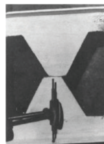
Fig. 4. Rupture of a welded joint (Halleux, 1967).
