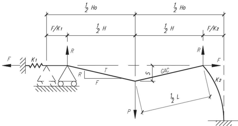
Fig. 3. HLL with elastic horizontal supports.
