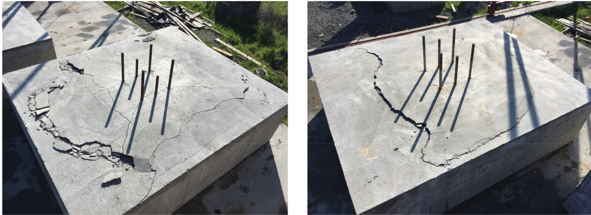
Fig. 5. Overhead view of breakout surface: (a) 12-in. embedment; (b) 18-in. embedment.
