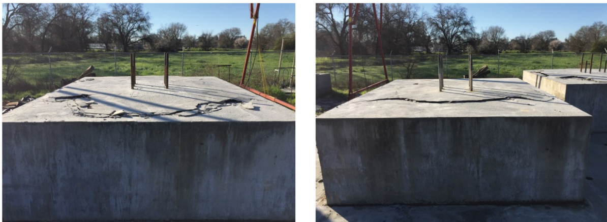
Fig. 6. Profile view of breakout surface: (a) 12-in. embedment; (b) 18-in. embedment.
