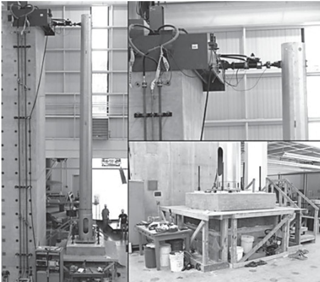
Fig. 10. As-built specimen test set-up (similar for all other specimens).
