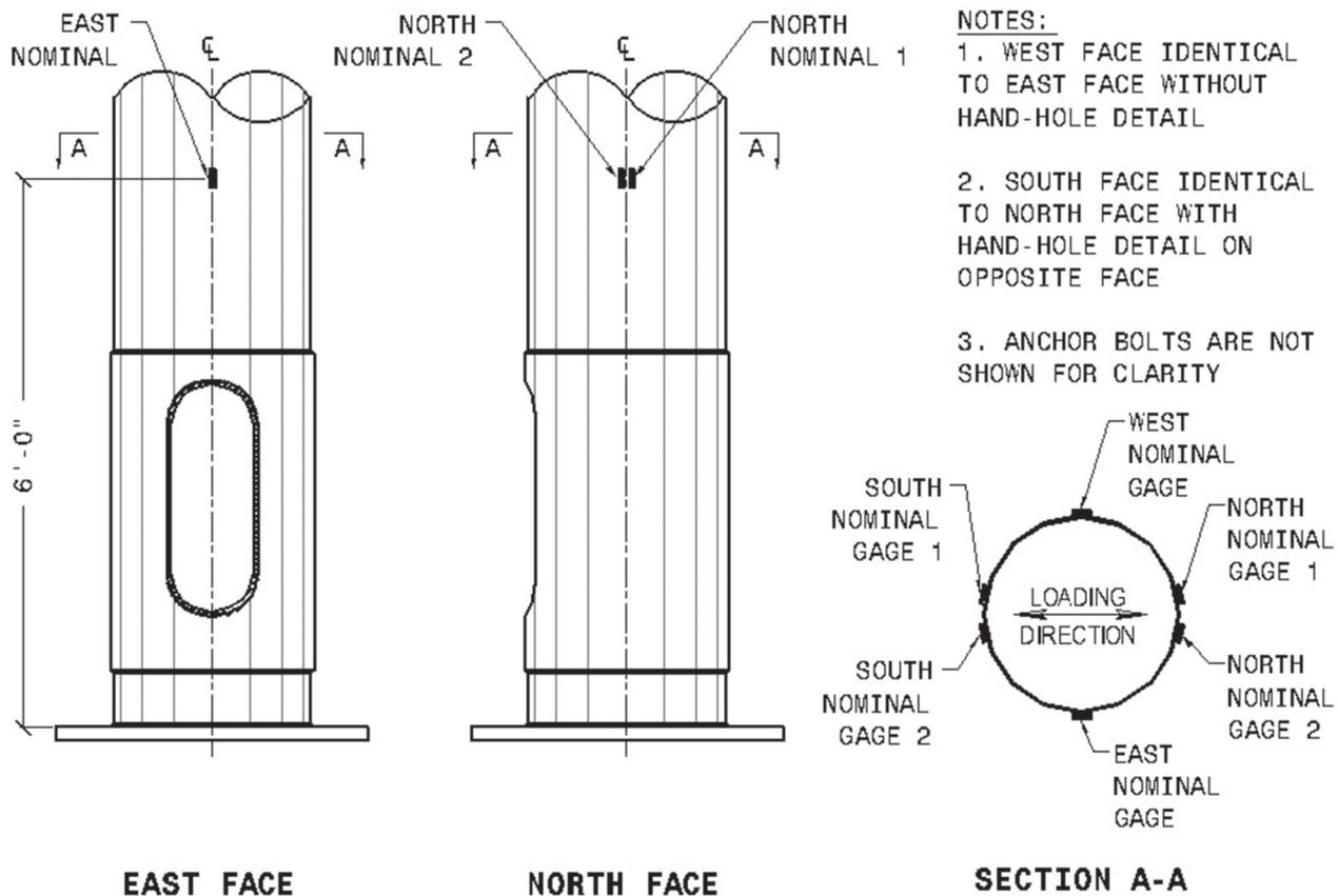
Fig. 2. Strain gage layout for as-built specimen.
