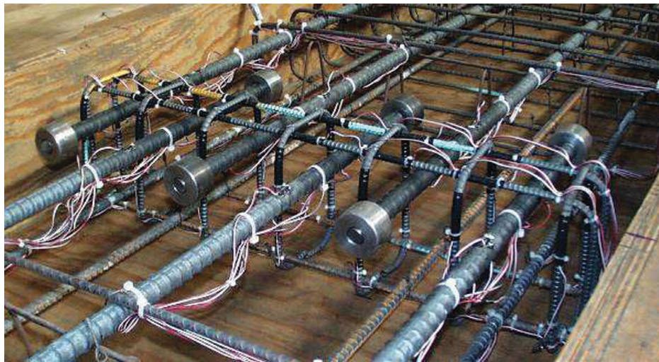
Fig. 23. Headed bar detail.
