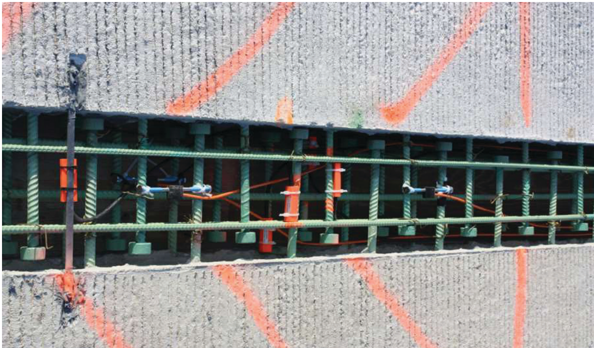
Fig. 26. Strain gages of closure in region 1.
