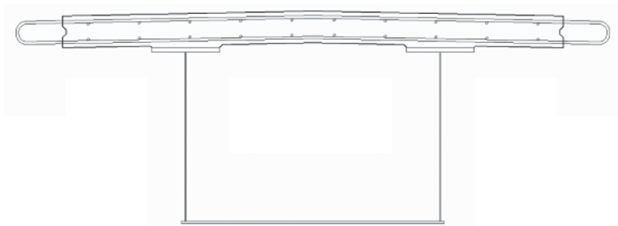
Fig. 14. Single (interior) box girder and deck unit.
