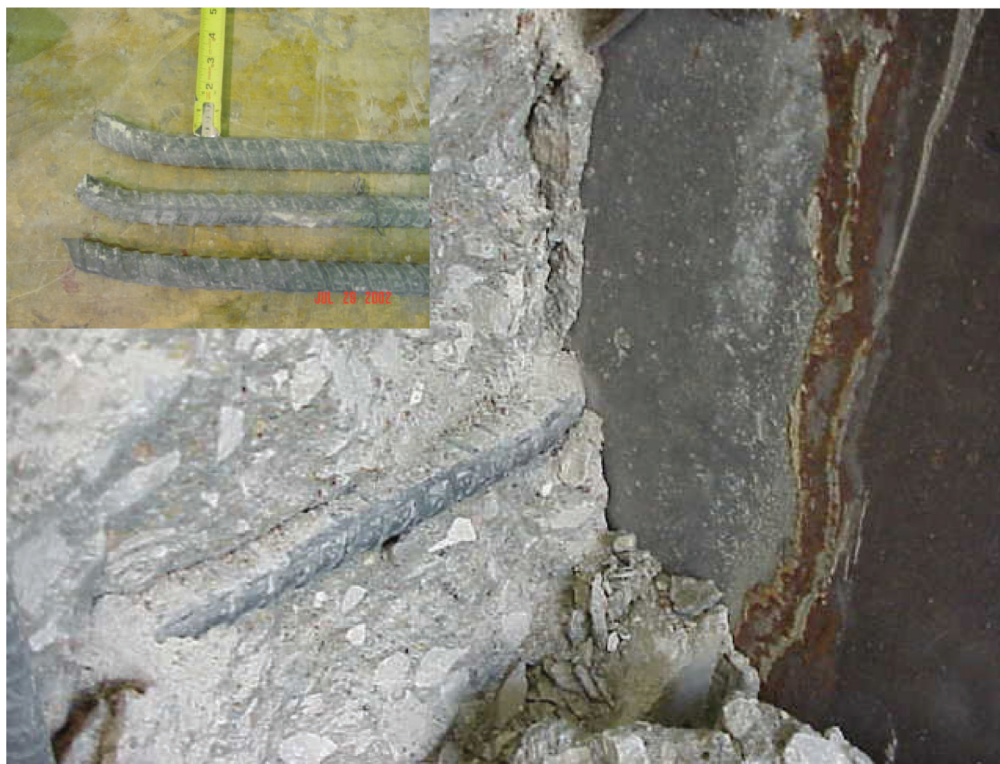
Fig. 23. Shear failure of the transverse bar inside the diaphragm after the conclusion of the ultimate test—specimen 2.
